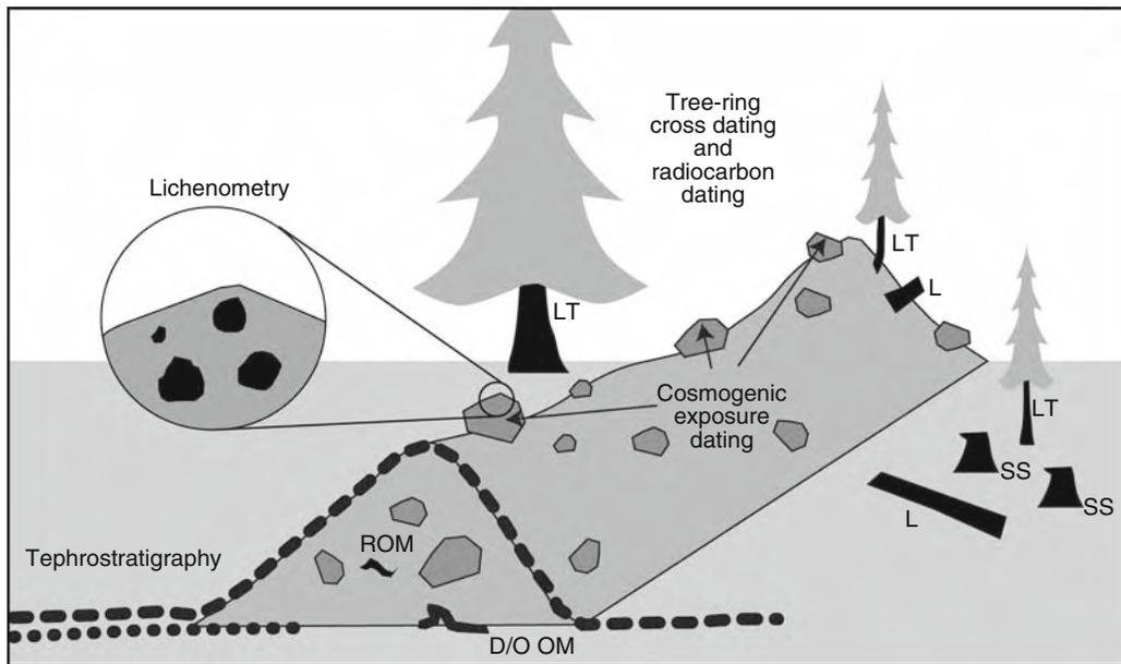
**Dating Glacial Landforms, Figure 1** Common methods used to date moraines. Targets for radiocarbon and tree-ring cross dating are labeled: *LT* living tree, *L* log, *SS* sheared stump, *ROM* reworked organic material, *D/O OM* deformed/overridden organic material. *Dashed and dotted lines* represent tephra layers.
