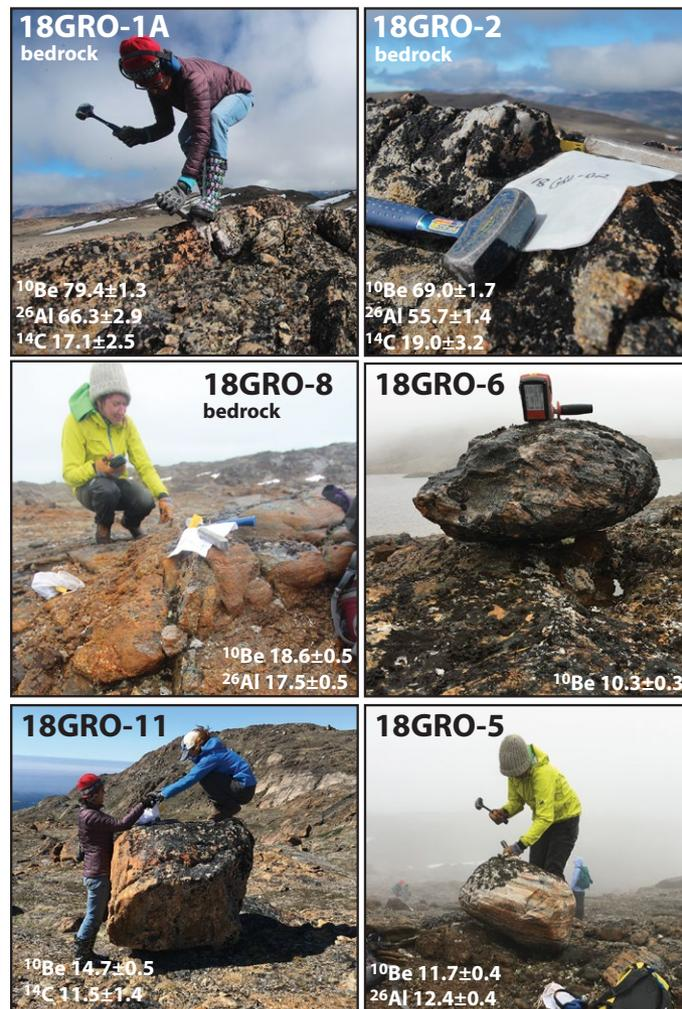
Figure 5. Photographs of selected samples show cosmogenic nuclide exposure ages and one standard deviation error (in ka).
