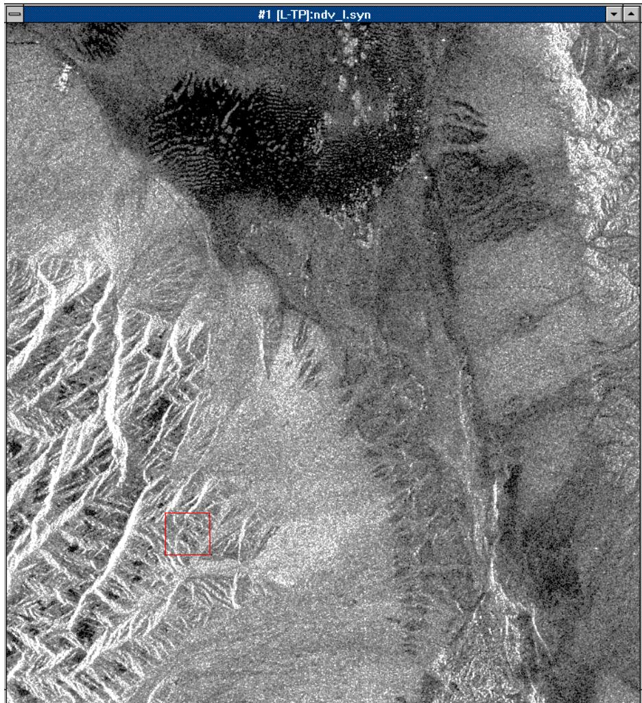
Figure 25-3: L-Band SIR-C Total Power Image with Gaussian stretch applied.
