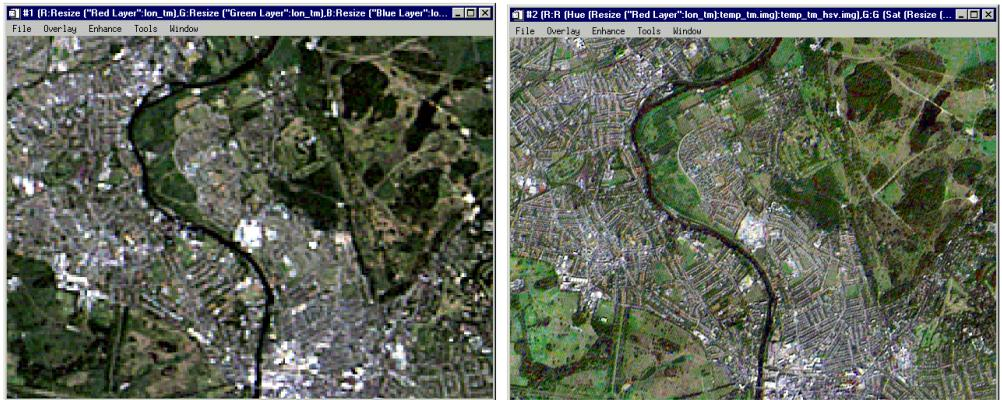
Figure 8-2: Landsat TM data (30 m spatial resolution, left). Fused Landsat TM and SPOT Panchromatic data (10 m spatial resolution, right).
