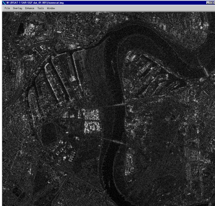
*Figure 24-3: Radarsat Image with Square Root Contrast Stretch Applied*
